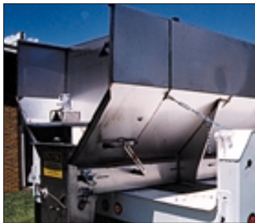
AC1420A Hydraulic drive, 3-Yard, 304 Stainless Steel Body.
